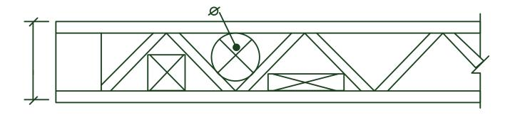
Plumbing, electrical and HVAC systems can be installed around and through open web area of the floor trusses.
