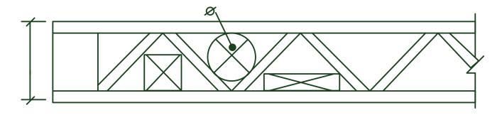
Plumbing, electrical and HVAC systems can be installed around and through open web area of the floor trusses.
